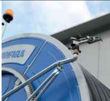
Second sprinkler on the machine frame
