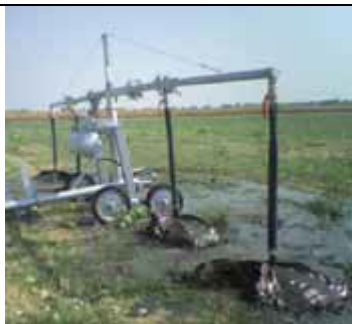
Boom for waste water
