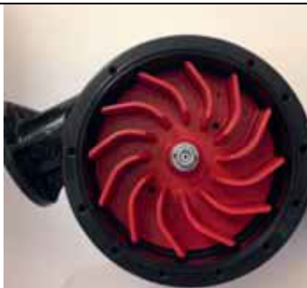
Turbine PLASCOAT painting
