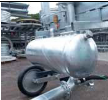
Water-ballasting tank for trolley
