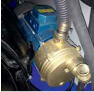
Self-priming electric pump
